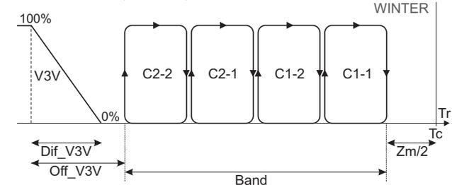
For the regulation of the hot water coil, the control has a proportional or on/off output Y2 which controls the three-way valve, and for the regulation of the electrical heaters, there are two on/off outputs NO6- NO7.
