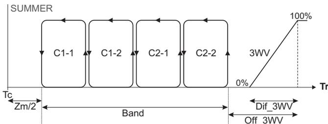
As backup cooling, these units can incorporate a cold water coil (V3V). For the regulation of the coil, the control has a proportional or on/off output Y2 which controls the three-way valve.
