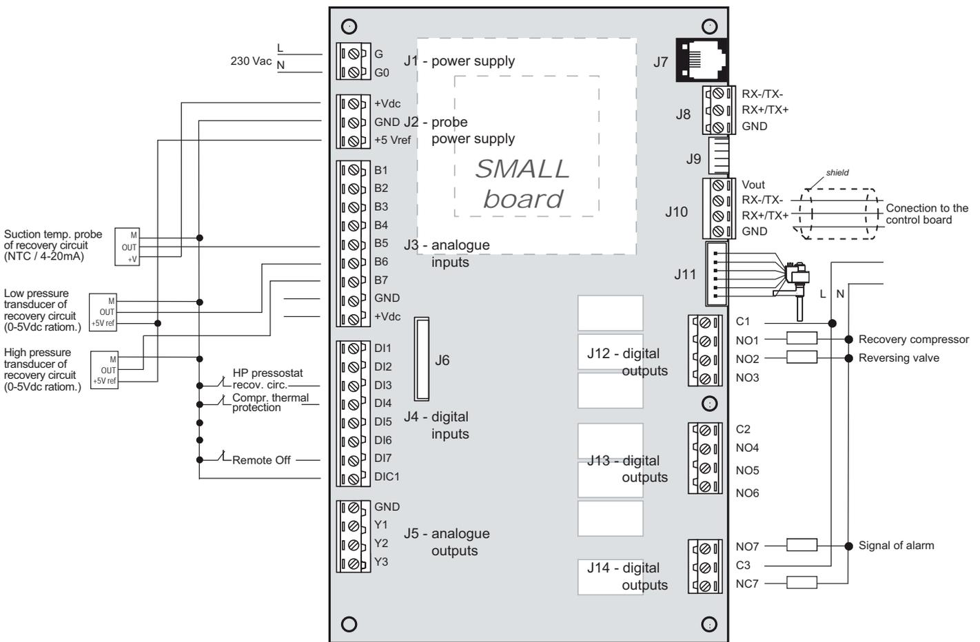
The management of the cooling circuit for the recovery of the extracted air energy (optional) is done with a SMALL board connected in series on the Field-Bus. Address 4.
