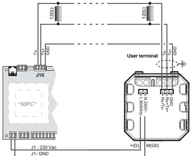
**Important:** It is recommended to insert an electrical resistance of 120Ω, between connectors TX+ and TX- of the board output (connector J10) and on the final component of the RS485 network, to avoid potential problems of communication.
