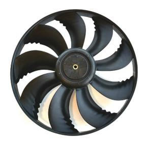
The 30XBEZE and 30XBPZE utilize Carrier's 6<sup>th</sup> generation Flying Bird<sup>™</sup> fan technology, engineered for maximum efficiency, super low noise, and wide operating range. The fan includes Carrier patented rotating shroud technology and back-swept blades with a unique wave-serration trailing edge inspired from nature.
